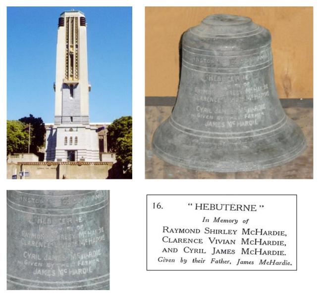
The Hebuterne bell is 28cm high and 34cm in diameter and had the musical pitch F3. Salt air exposure and attendant corrosion has unfortunately caused this bell to go progressively flat and lose its pitch. In 1985 it was replaced and the original put into storage at the National War Memorial as an historical artefact.
